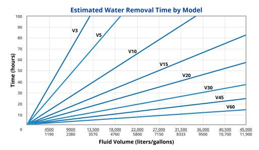
No other technology removes water faster or more safely with less chance of foaming than the Hy-Pro VUD. The graph here represents the estimated time required per model to remove water from 5000 ppm (0.5%) down to 150 ppm (0.015%) for increasing reservoir sizes.
