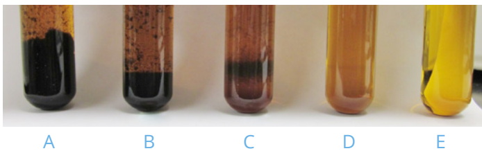
Figure 1 – Deposition Tendency Test
